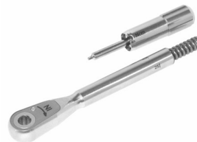
Fig. 2 Unscrew completely the torque adjustment screw (7) and extract the spring/stop (6).
