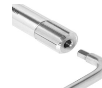
Fig. 8 The assembly of the torque wrench is complete as soon as the spring/stop is in place and the torque adjustment screwed back in the handle. Check the function by activating the ratchet wheel. If there is a regular ratchet noise, the instrument operates correctly. Before use, always check the assembly and the correct function of the torque wrench.
