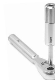
Fig. 7 Once the parts (1) and (2) are in place, put the cover (3) on the ratchet head (4) and adjust. Turn the torque wrench while holding the cover. Fix the screw (5) tightly with the hexagon shank bit (7) of the torque adjustment screw.
